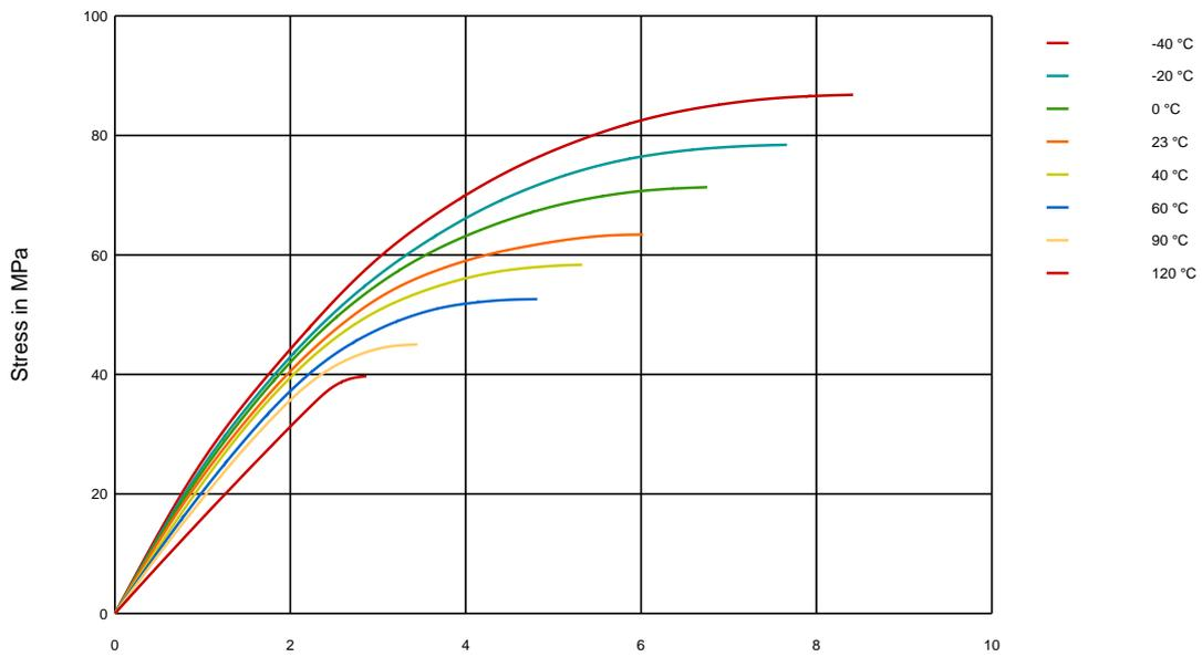
Fig. 2: Isothermal stress-strain curves from the short-time tensile test to ISO 527-1, -2 (Makrolon<sup>®</sup> 2405, 2407)
