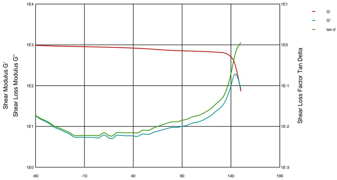
Fig. 3: Shear modulus as a function of temperature to ISO 6721-1, -2 (Makrolon® 2405, 2407)
