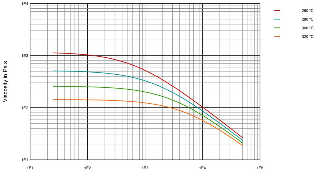
Fig. 1: Melt viscosity as a function of shear rate (Makrolon<sup>®</sup> 2405, 2407)
