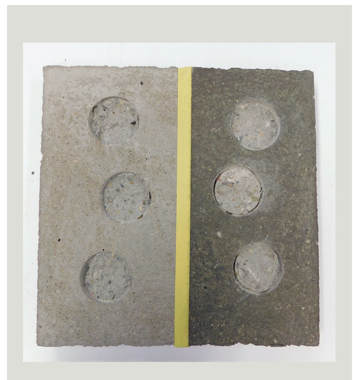
Figure 3: Cement screed panel coated with 2C-PAS primer after determining adhesive tensile strength.
